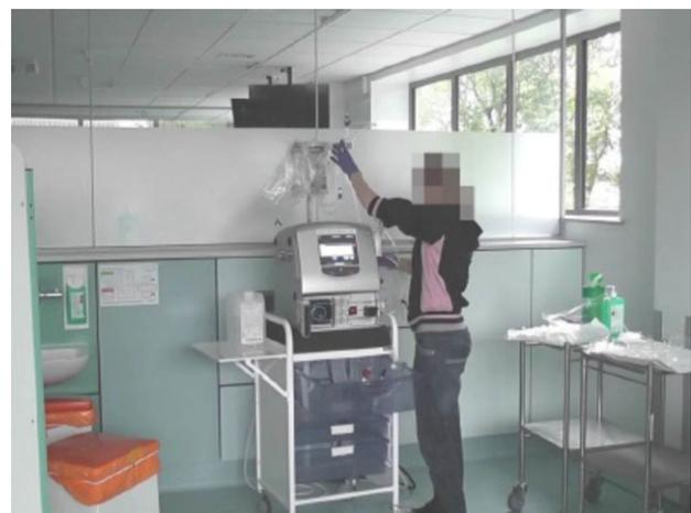
**Figure 2** Test room set-up for Human Factors Testing of the Quanta SC+ home hemodialysis system [Color figure can be viewed at [wileyonlinelibrary.com](http://wileyonlinelibrary.com)]
