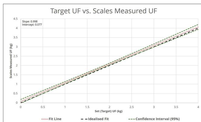
Figure 1: Target ultrafiltration on SC+ plotted against the actual fluid removed by weight change pre- and post-treatment.
